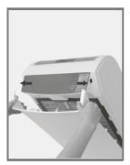
Open the front filter flap and then remove all filters
